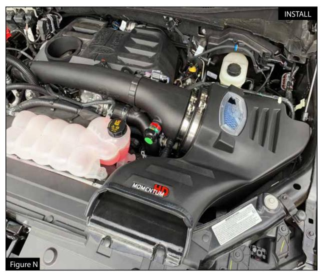
Refer to Figure N for Steps 27-28 Step 27: Reconnect the negative battery terminal. Step 28: Verify all clamps and screws are secure. Your installation is now complete. Thank you for choosing aFe POWER!
